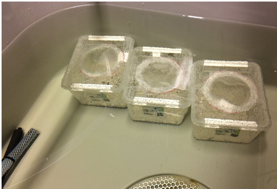
FIGURE 1 Schematic representation of the experimental setup of Test I. Each box represents a tank with submerged cages, and each cage contained a given number of specimens of a single species. The treatment groups (T) were exposed to total dissolved gas (%) according to the number in their name. Tests II and III were implemented in a similar manner. The lower image shows the T115 tank from Replicate 2 with submerged cages.
