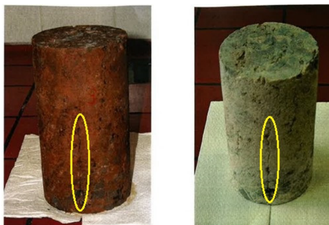
Figure 3. Images of whole diameter core from the Vranovice carbonate formation for well ZA4A; depth: 1781–1781.3 m. The (left) image displays a core sample before and (right) image after cleaning and drying. Fracture located in the core is marked in yellow.
