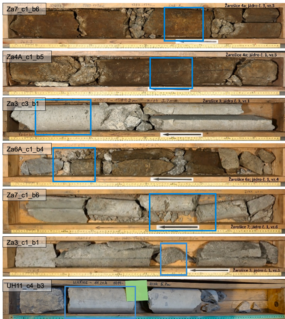
Fig. 1. Picture of the samples acquired from the storage repository. The box number is termed with the field, the well number, core number (jádro) and box number (vz). The blue rectangles depict the samples used in the geomechanical analysis.
