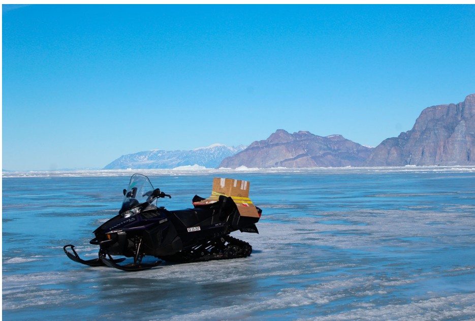
Figure 7. This snowmobile was incapacitated due to overheating on bare shorefast ice in Uummannaq Fjord, May 2019. Lack of snow cover increases difficulty of snowmobile travel over shorefast sea ice. Credit: S. Cooley.
