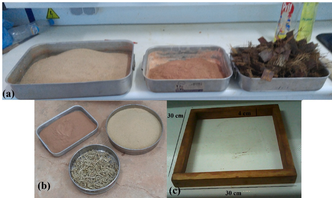
Fig. 1. Picture of composite sample: (a) Sand, clay, and date palm fibers; (b) Sand, clay, and date palm spikelet; (c) Mold dimensions.
