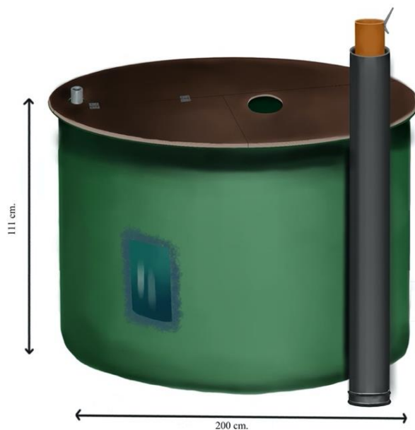
Figure 3 The schematic of the housing tanks. The housing tanks had a dimension of 111 cm height and 200 cm diameter. Water depth was 85cm.
