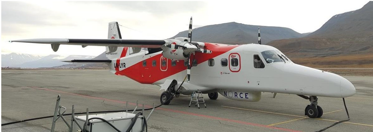
Figure 2 Lufttransport's Dornier DO-228 aircraft (LN-LYR). The optical instrumentation and communication payload are installed in the pod towards the front of the aircraft.
