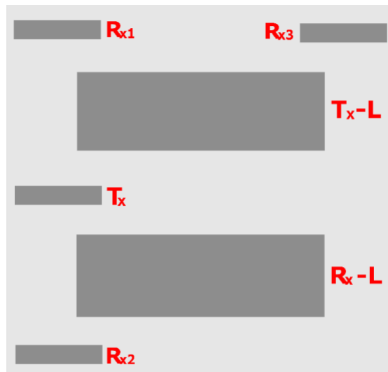
Figure 7 : Candidate X-, and L-band antenna configuration on the Dornier at the rear part of the aircraft.
