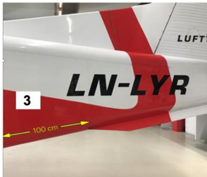
Figure 4 : An approximately 1 m x 1 m space is available for mounting the antennas at the rear part of the aircraft.
