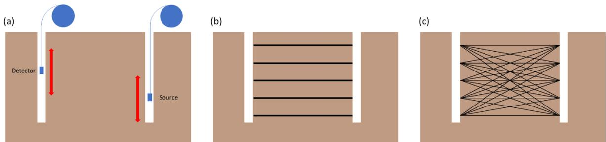
*Figure 2. a) Schematic setup for conventional borehole seismic experiments. b) Seismic ray path defining source and detector positions for conventional cross-well experiments. c). Seismic ray paths defining source and detector positions for conventional borehole tomography experiments.*
