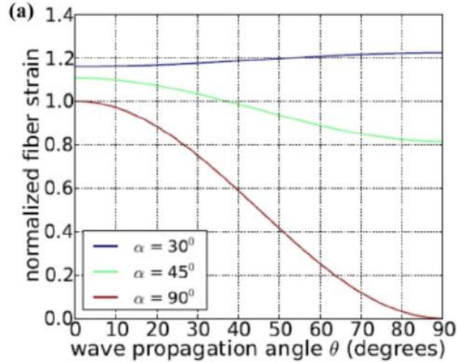
Figure 4) P-wave sensitivity function for a helical fibre for different helical fibre wrapping angles,  $\alpha=90^\circ$  corresponds to a straight fibre. (Kuvshinov 2016)
