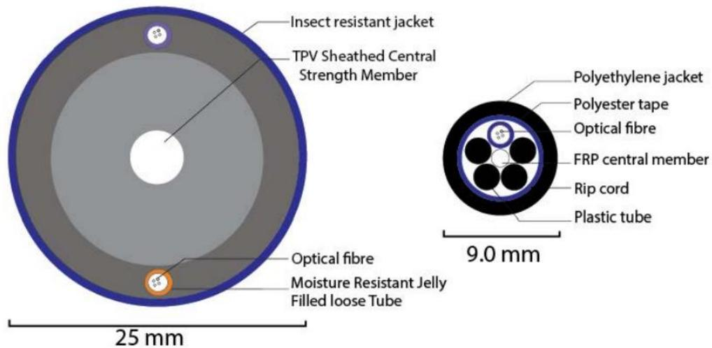
Figure 7) Structure of the helical (left) and straight (right) cables installed at Svelvik.
