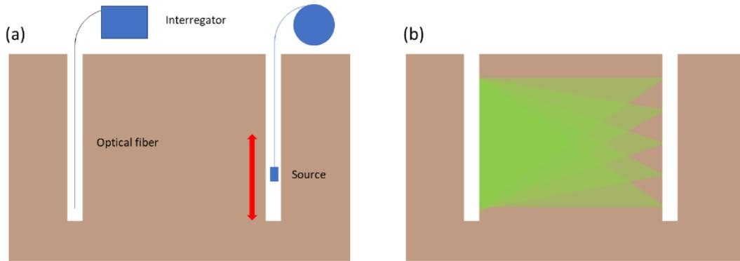
Figure 3 a) DAS cross-well seismic configuration b) Detectable seismic ray paths tomography measurement made using a distributed acoustic sensor. When using a distributed fiber, only the source position needs to be changed.
