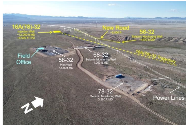
Figure A1. Photo of FORGE site. Currently existing wells are white, planned in yellow. From https://utahforge.com/data-dashboard/current-and-planned-activities/
