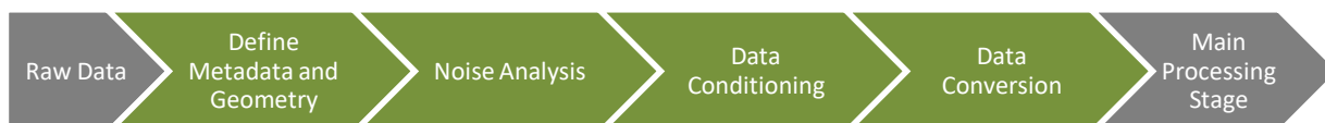
Figure 11. Preprocessing workflow comprising of four stages to prepare the raw seismic data for the main processing stages.
