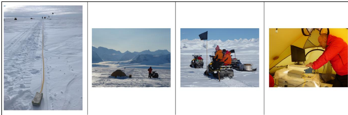
Figure 2. Field deployment photo at Rutford Ice Stream (BEAMISH), left to right: the linear array with a distant flag marking one of the Reftek/geophone stations (station A000); the recording tent – the petrol generator was located 50m from the tent; ploughing a furrow for the cable; inside the recording tent.
