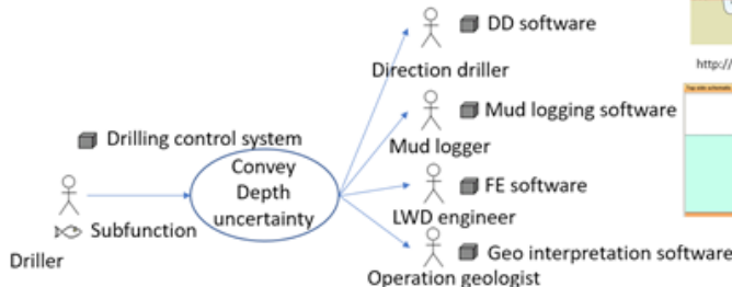
Fig. 4—Example of use case for vertical datum reference. Here, DD, LWD, and FE stand, respectively, for directional drilling, logging while drilling, and formation evaluation.
