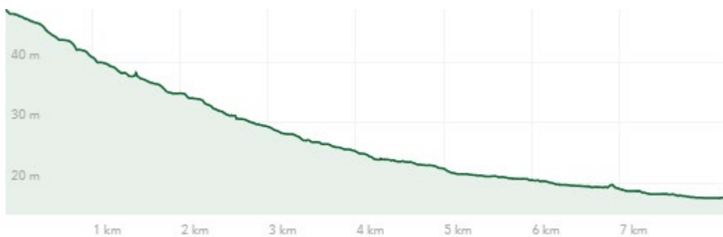
Figure 30: Longitudinal profile of river Bøelva.
