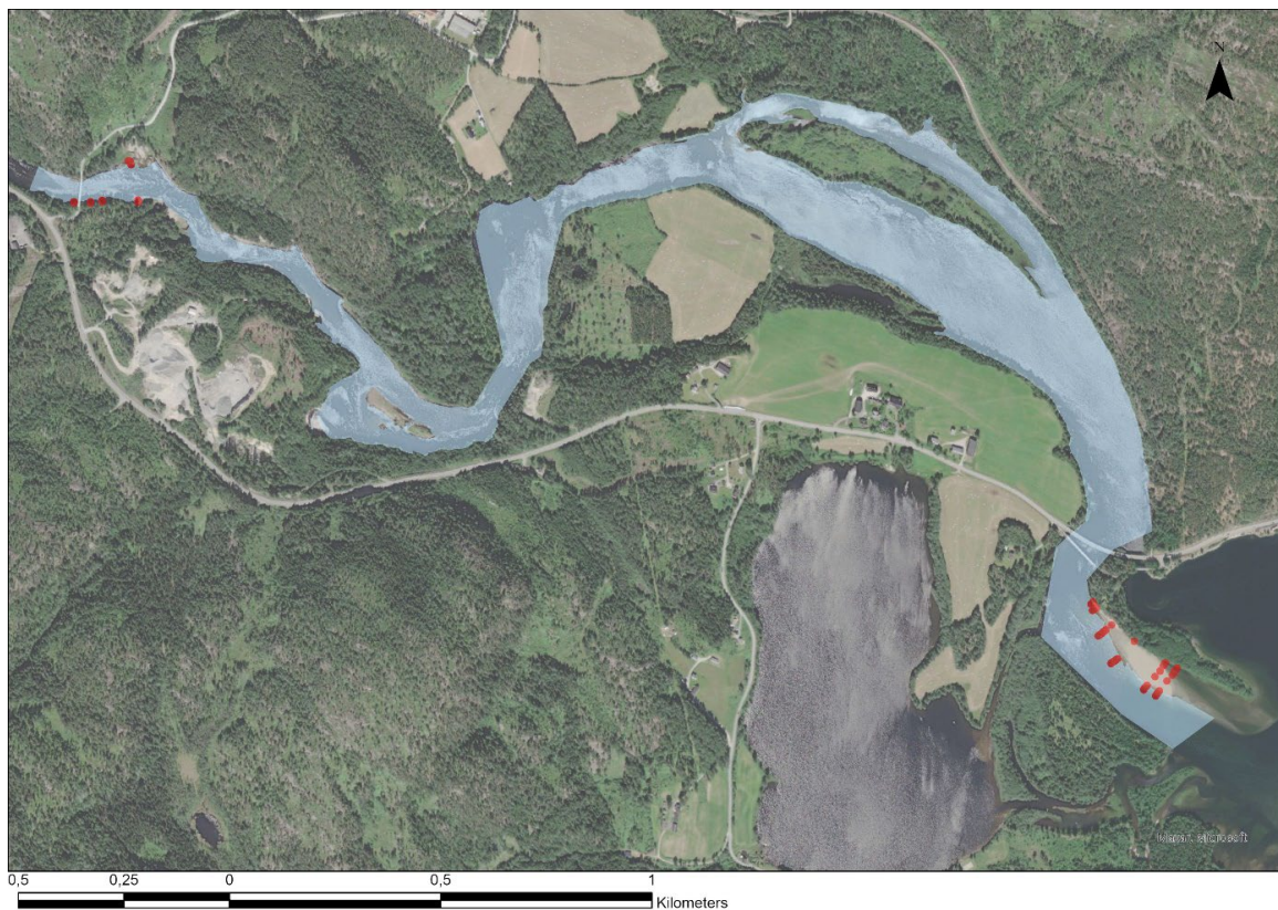
Figure 5: Overview over the mapped stretch in river Hallingdal, manually surveyed cross sections marked in red, scanned area in blue.
