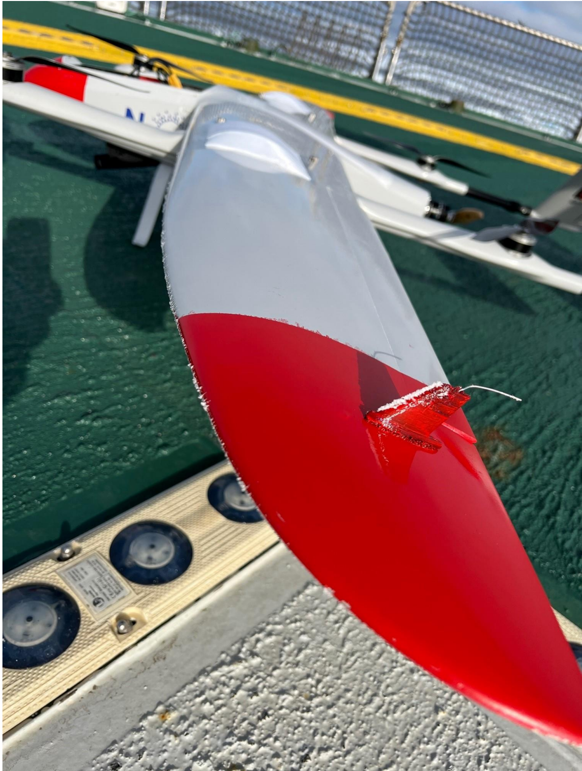
Picture 6: Ice on Cryowing Fox during CIRFA cruise in Fram strait 2022 (Photo: Andre Kjellstrup, NORCE)
