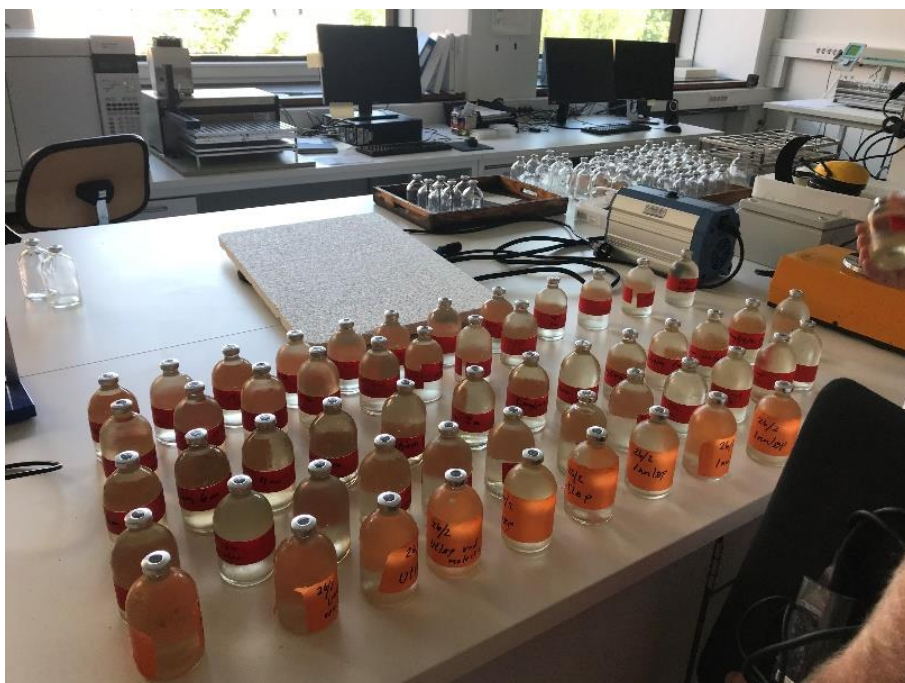
Fig. S2. Water samples warming up to lab temperature before creation of a helium head space for the gas chromatograph. NMBU, Ås. Photo: Benoît Demars/NIVA.
