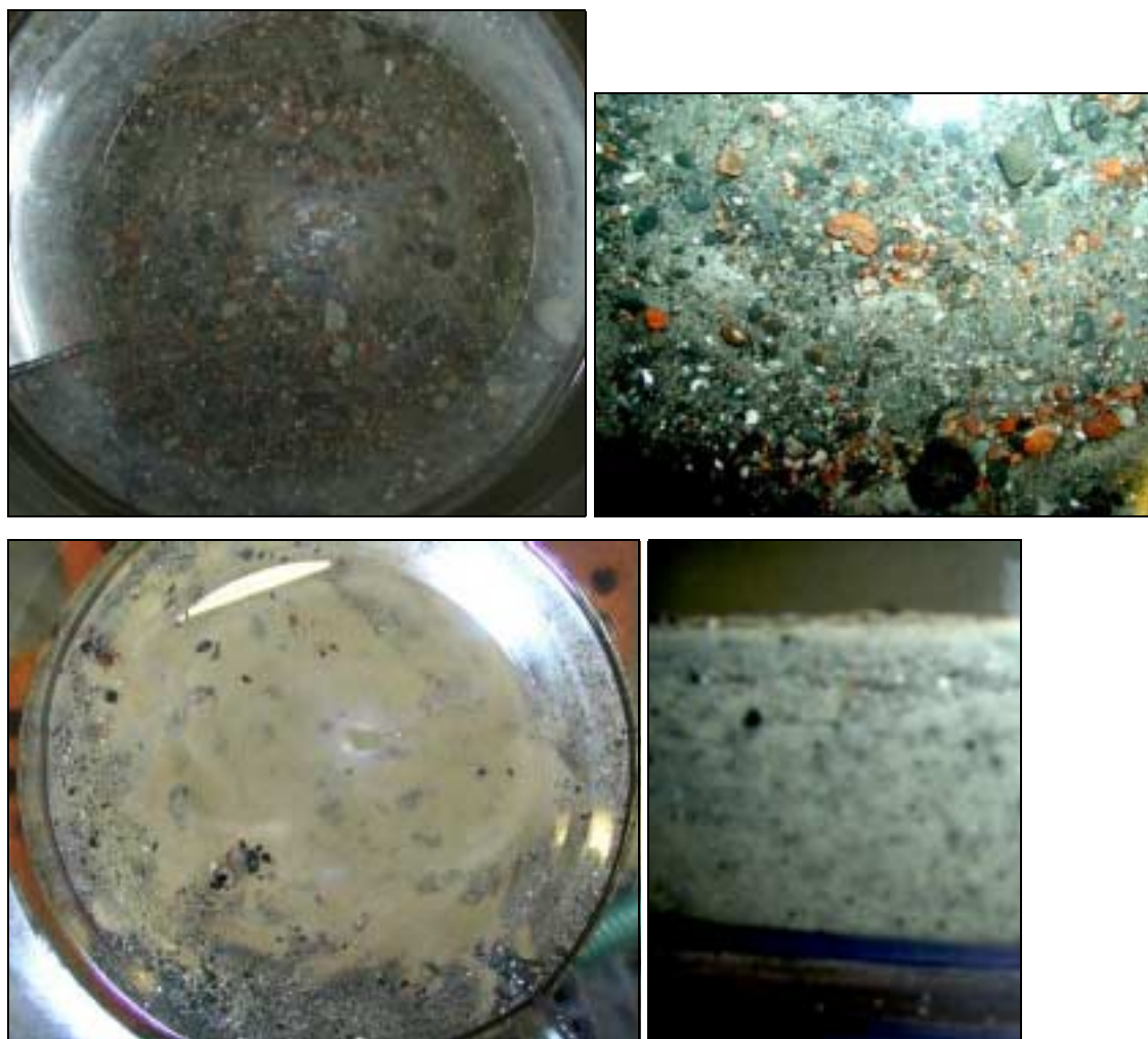
Figure 6. Top: Photographs of Beryl cuttings (“Much disturbance”) viewed from top of chamber at the end of the experiment 28 th August (flash reflex masked) and close-up (upper right, colour and contrast modified). Below: Beryl cuttings (“No disturbance”) viewed from top of chamber (flash reflex masked) and from side (28 August). Note the difference in top layer, with more coarse particles on top in the ‘much’ treatment, and smaller particles in the top layer of the ‘none’ chamber (no disturbance). Side view (below, right) indicates darker spots in the sediment.
