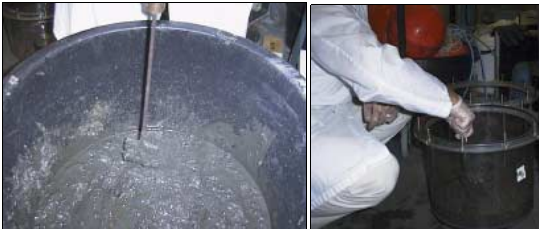
Figure 1. Homogenisation of Beryl cuttings (left) before transferring it to the test chambers (right).
