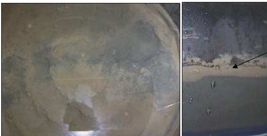
Figure 5. Photos of Ekofisk cuttings (“Little”) from top (flash reflex masked) and side of chamber (25 June). Both photos indicate a brighter surface (3-5 mm thick, see arrow) with darker (lower Eh) sediment below. The rake had recently been turned 1/10 and removed (se marks on surface).
