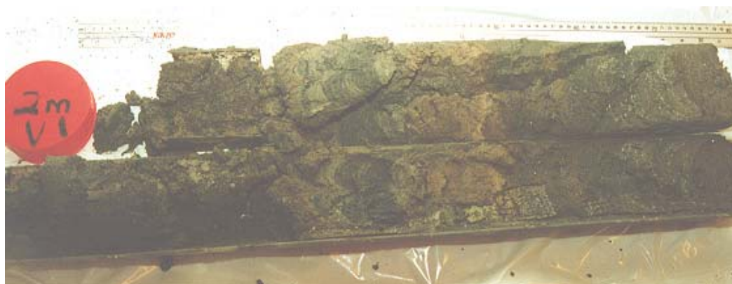
Figure 4: Lower part of vibrocore 1 (V1) from Beryl. The layering seen on the picture corresponds to the layers into which the cores were divided for further analysis.
