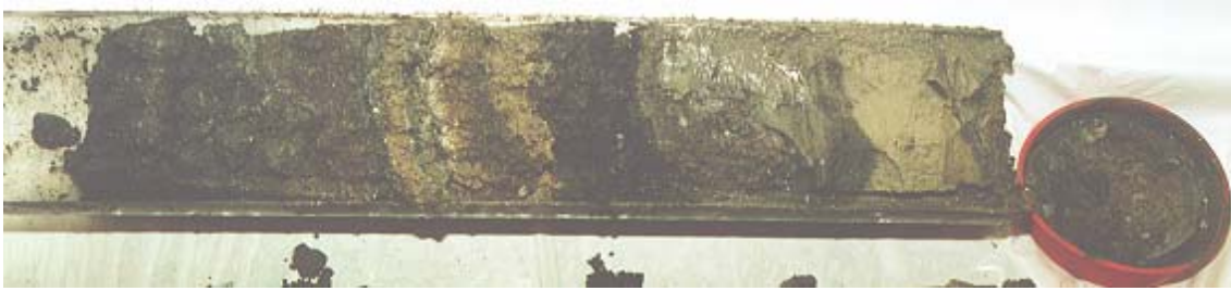
Figure 5: Sub-core (SW3) from a box corer taken at Ekofisk 2/4A. The layering seen on the picture corresponds to the layers into which the cores were divided for further analysis.
