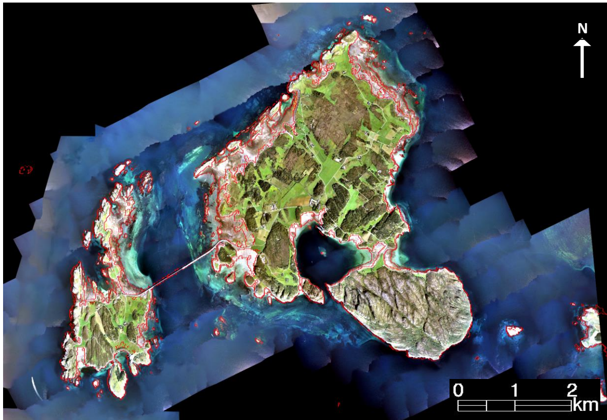
Figure 21. Detected intertidal zone area (red) superimposed on an aerial image from Storfosna.
