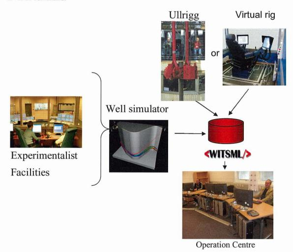
eLAD shall provide an environment which replicates as accurately as possible the context for decision making during drilling operations. The laboratory is therefore including a rig site where a drilling crew can perform the drilling operations and an operation centre where data can be analyzed. The rig site can either be Ullrigg which provides a full size drilling rig equipped with modern drilling machineries and a top of
