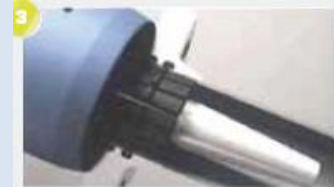
3 Hydraulic tool extrudes pipe into grooves.
