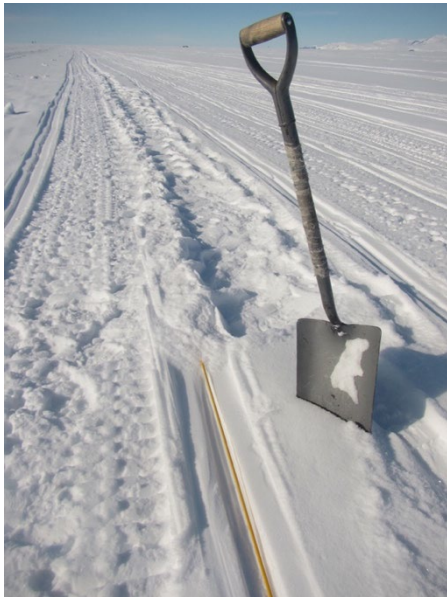
Figure B1. A photo of covered and uncovered portions of the fibre. Even a surficial cover of snow made a significant difference to noise levels.
