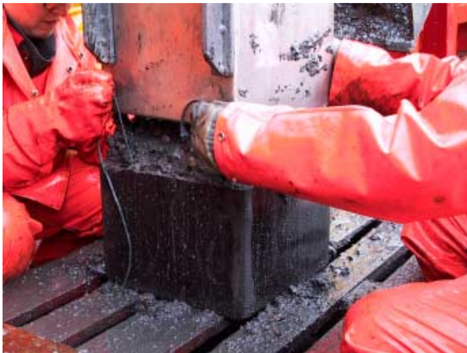
Emptying the box-corer into the plastic boxes specially designed by SINTEF to obtain undisturbed samples for erosion experiment
