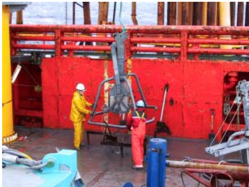
The box-corer being aligned in the rack onboard the ship. The rack was specially designed to efficiently collect bulk material for the other tasks in this UKOOA project.
