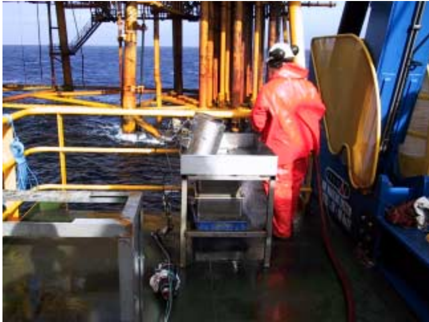
The van Veen Grab on the sciving table for the Benthos samples
