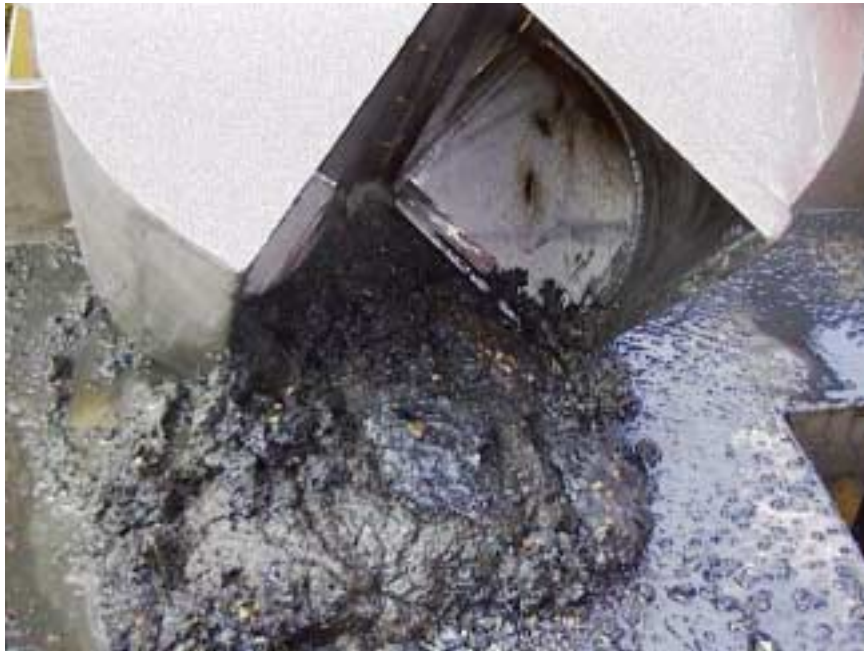
The van Veen with a sample. The van Veen Grab worked excellent in the cuttings pile. To get samples up to 10 cm thick for any type of purpose this is the simplest and most efficient tool to use
