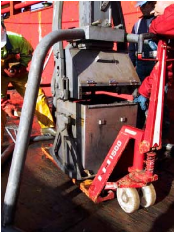
Removing the box to be able to take sub cores from the box-corer.
