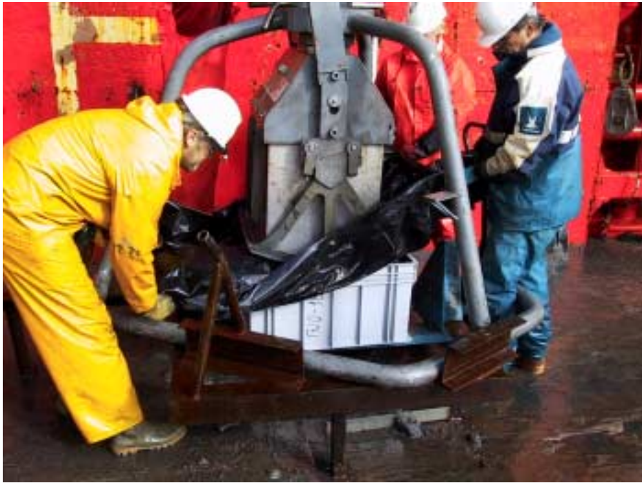
Emptying the box-corer into the plastic boxes where the bulk material was collected.
