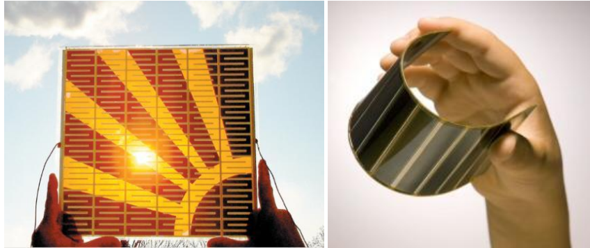
Figure 20: Examples of dye-sensitized solar cells. Source: Fraunhofer ISE, Germany.
