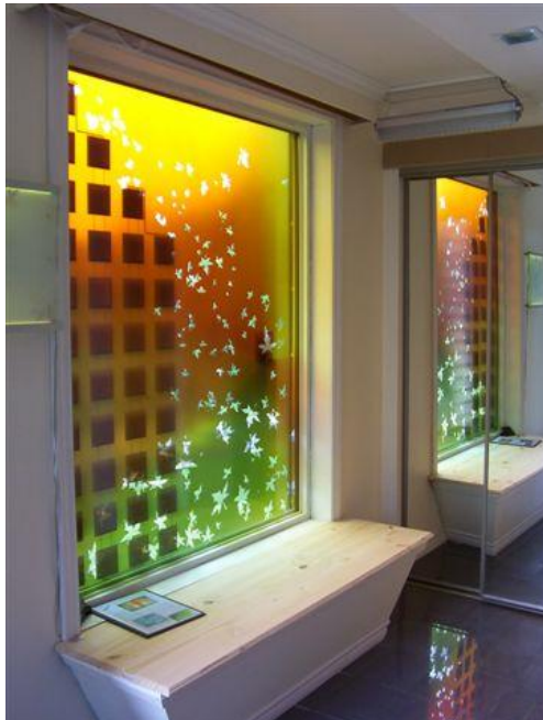
Figure 42: Solar cells embedded in colored glass, from Atlantis Energy Systems ( http://atlantisenergy.com ).
