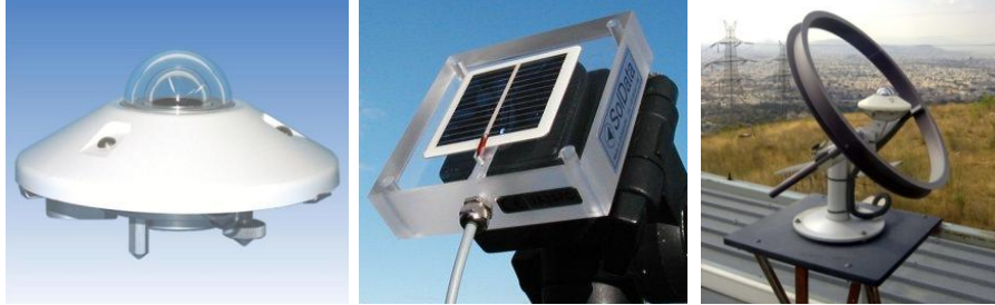
Figure 13: Measurements of irradiation can be done by pyranometers (right) or reference cells (middle). Using a shadow ring, the diffuse radiation can be measured with a pyranometer as shown in the right picture.
