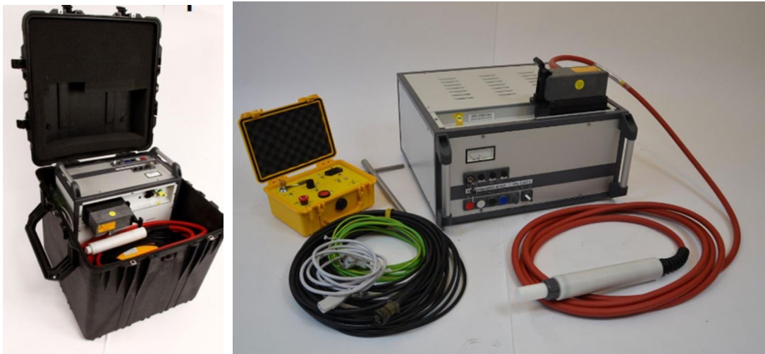
Figure 12: Impulse generator IPG and remote-control unit RCU
