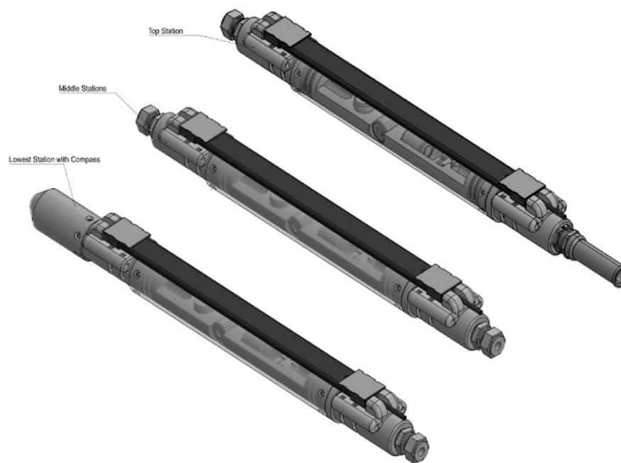
Figure 22: Components of re-designed Multistation Borehole Acquisition System (MBAS)
