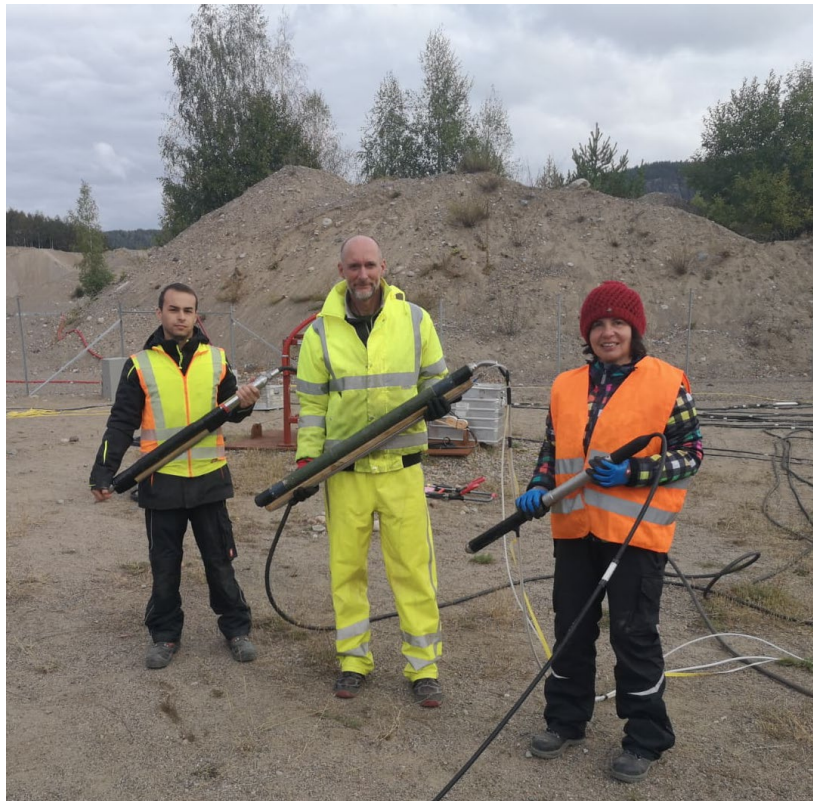
Figure 7: Three applied seismic sources (SBS42 right, BIS-SV middle and BIS-SH left)
