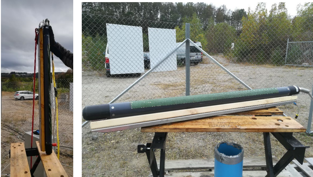
Figure 19: Prototyp of novel SV source BIS-SV
