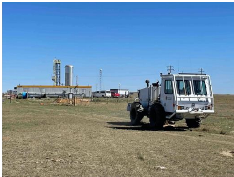
Figure 4. A mini-vibroseis source acquiring data at the Field Research Site (FRS) in Alberta, for the DigiMon project. The Field Research Site (FRS), a CO2 storage test site, is operated by Carbon Management Canada.
