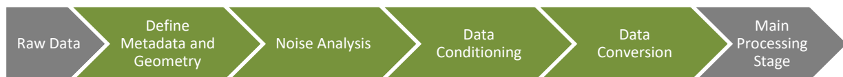
Figure 1: Preprocessing workflow comprising of four separate stages preparing the raw seismic data for the main processing stages.
