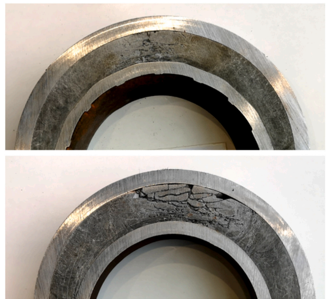
Fig. 19. Cross sectional view of the annular cement at the dent placed at 1.3 m in assembly C6 (top panel) and at 1.35 m, or 5 cm to the right of the dent (bottom panel).
