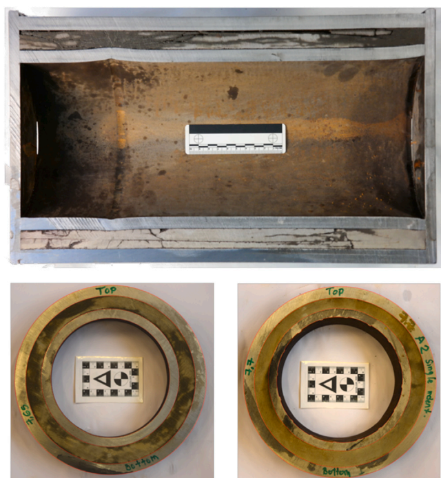
Fig. 10. Illustration of axial cut (top) and cross-sectional cuts (bottom) for assessing remediated annular cement.
