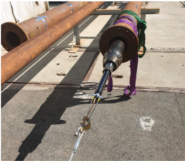
Fig. 7. The casing expansion tool partly inside one of the test assemblies. A dual winch system was used to position the tool inside the assemblies prior to each dent.
