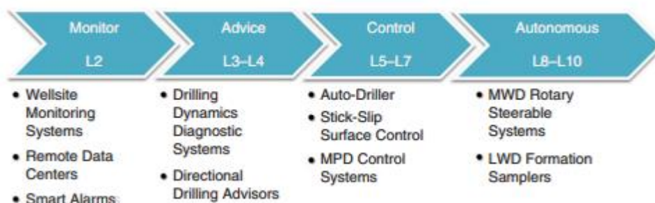
Figure 2: a classification of drilling automation systems, from (Macpherson J. D., et al., 2013).
