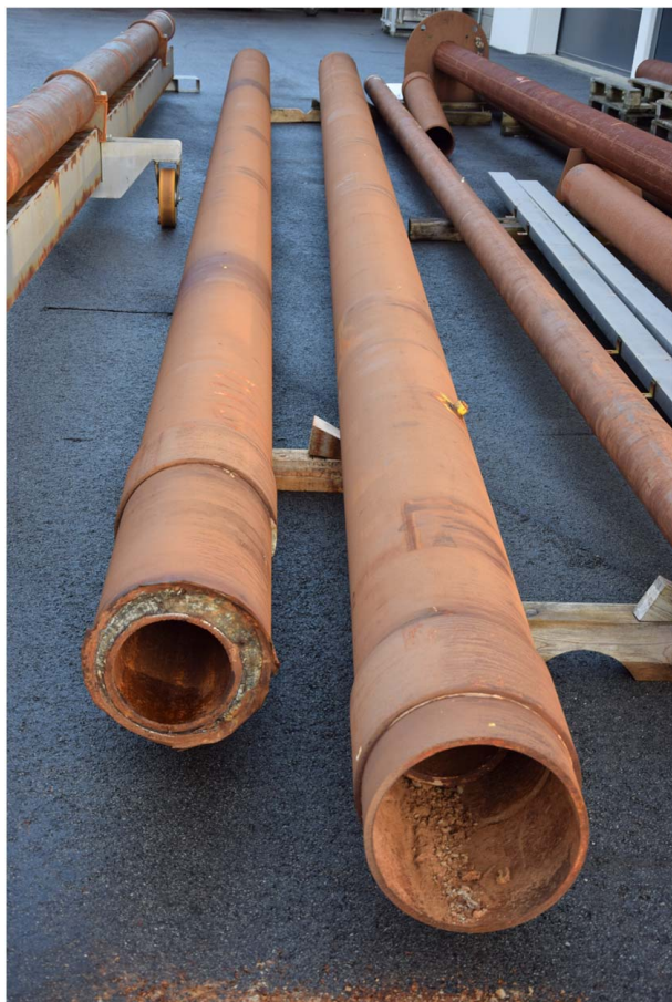
Fig. 3 Two cut and pulled sections from a North Sea well. The transition joint is shown to the right.
