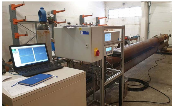
Fig. 1 The PWC Jig placed horizontally for pressure testing
