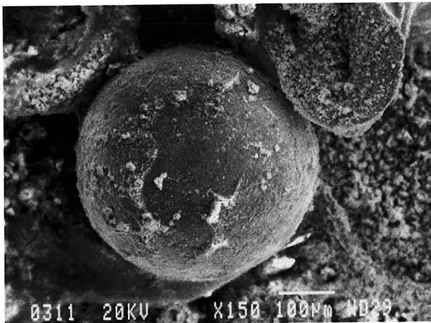
Figure A.17. SEM micrograph of a generic corrosion product; sampled from the pipe 3 months exposure (magn. 150X).
