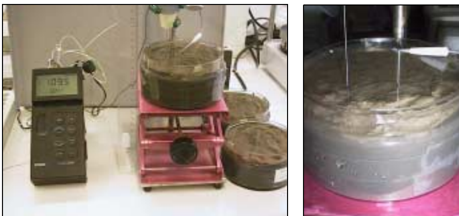
Figure 2.5 Set-up for redox and pH measurement. Detail to the right.
