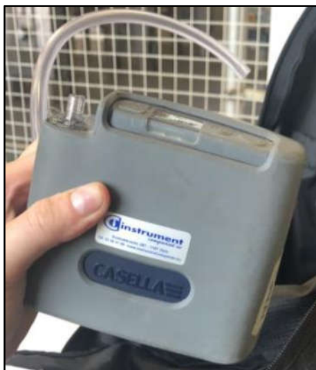
Figure 2 – Image of one of the Casella Apex2 personal sampling pumps used in the study. Credit: Geir Skoberbø, IVAR IKs
