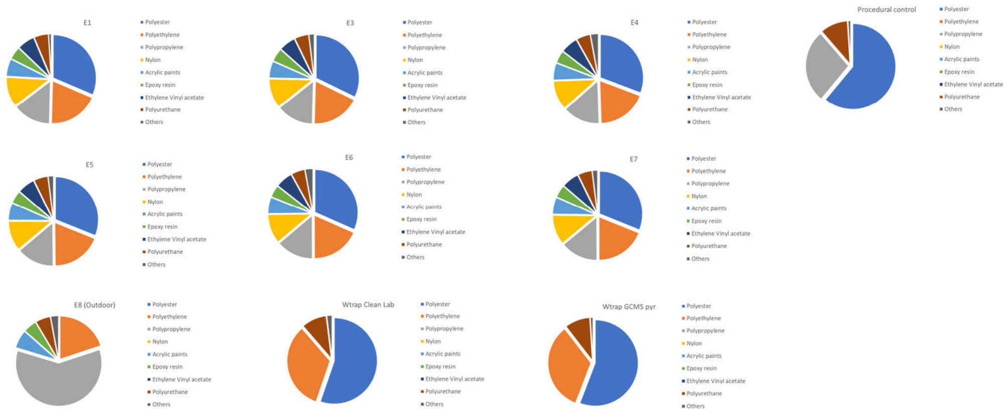
Fig. 9 – Pie charts of relative polymer distribution assessed by \mu -FTIR imaging analysis. The category “Other polymers” groups the polymers present in lower percentages (polyvinyl acetate, phenoxy resin cellulose acetate and triacetate, polylactic acid, polycarbonate).
