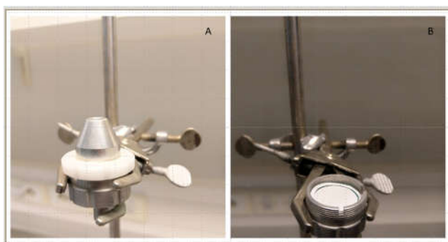
Figure 3 - Image of the aluminum sampling head (A) holding the 25 mm fiberglass filter (B).
