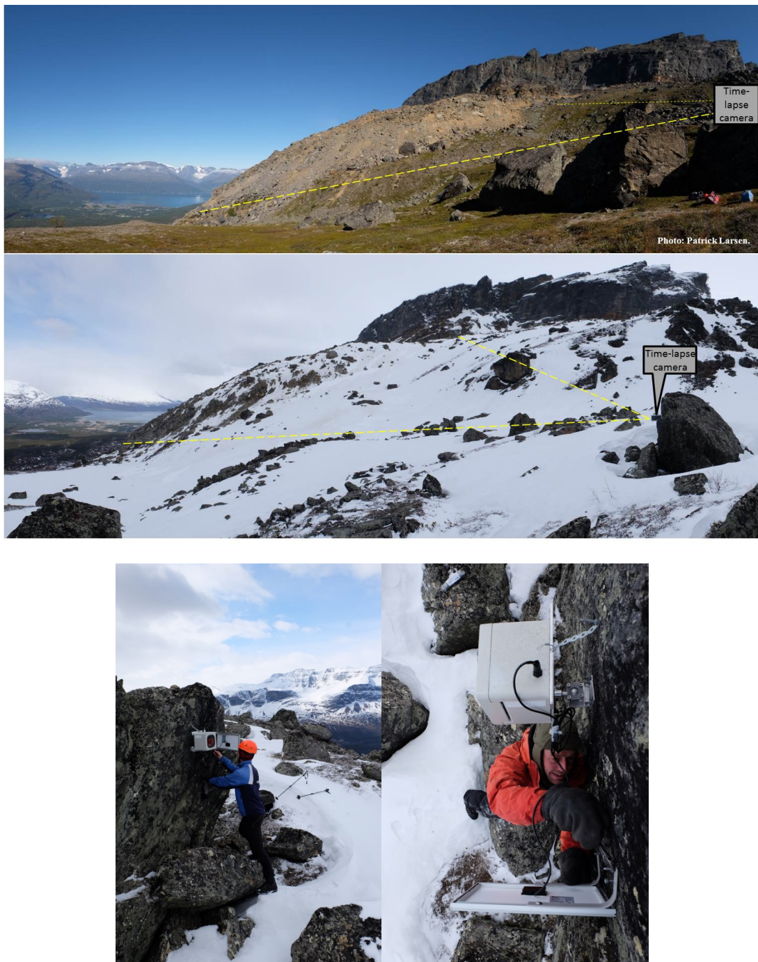
Figure 22 – Location, line-of-sight and setup of a time-lapse camera (TL CAM) overlooking the most active rock glacier lobe (NW) on Ádjet.
