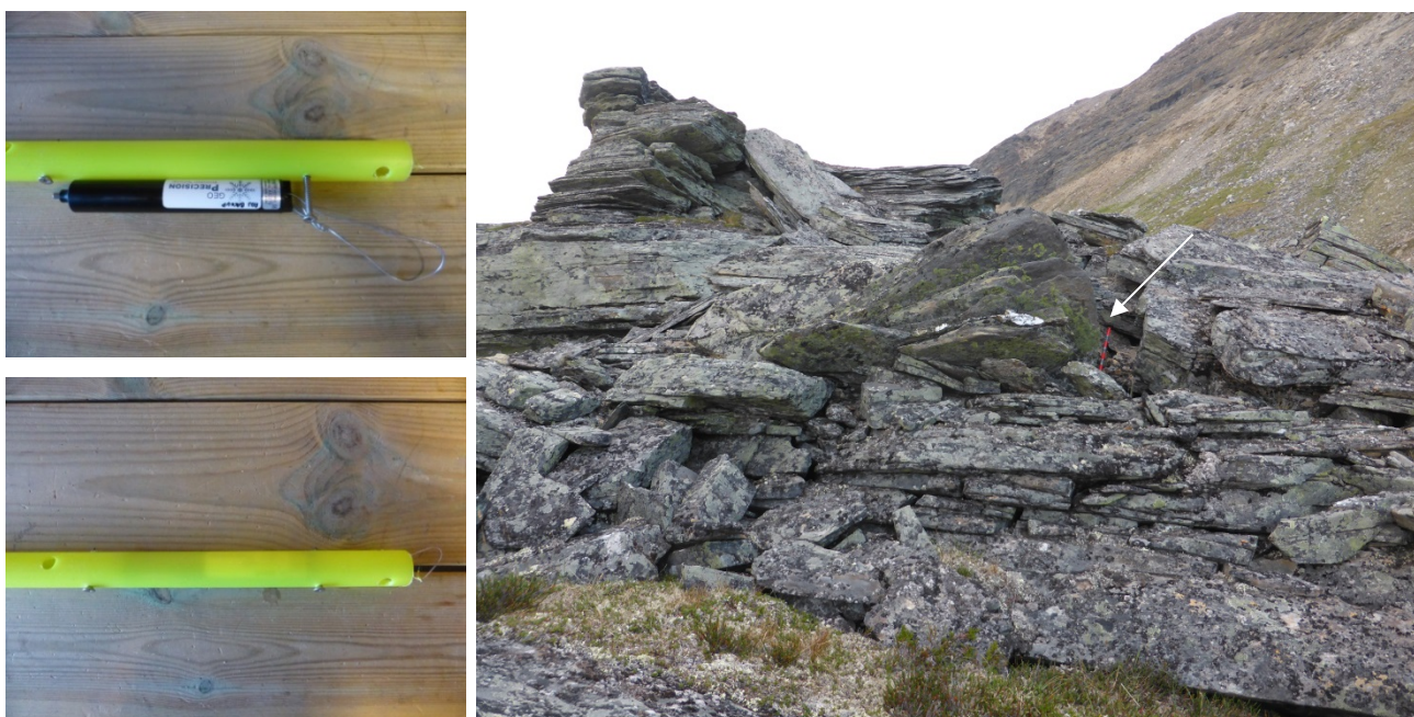
Figure 2 – Mounting of GeoPrecision loggers inside plastic sticks and examples of placement in space between boulders.
