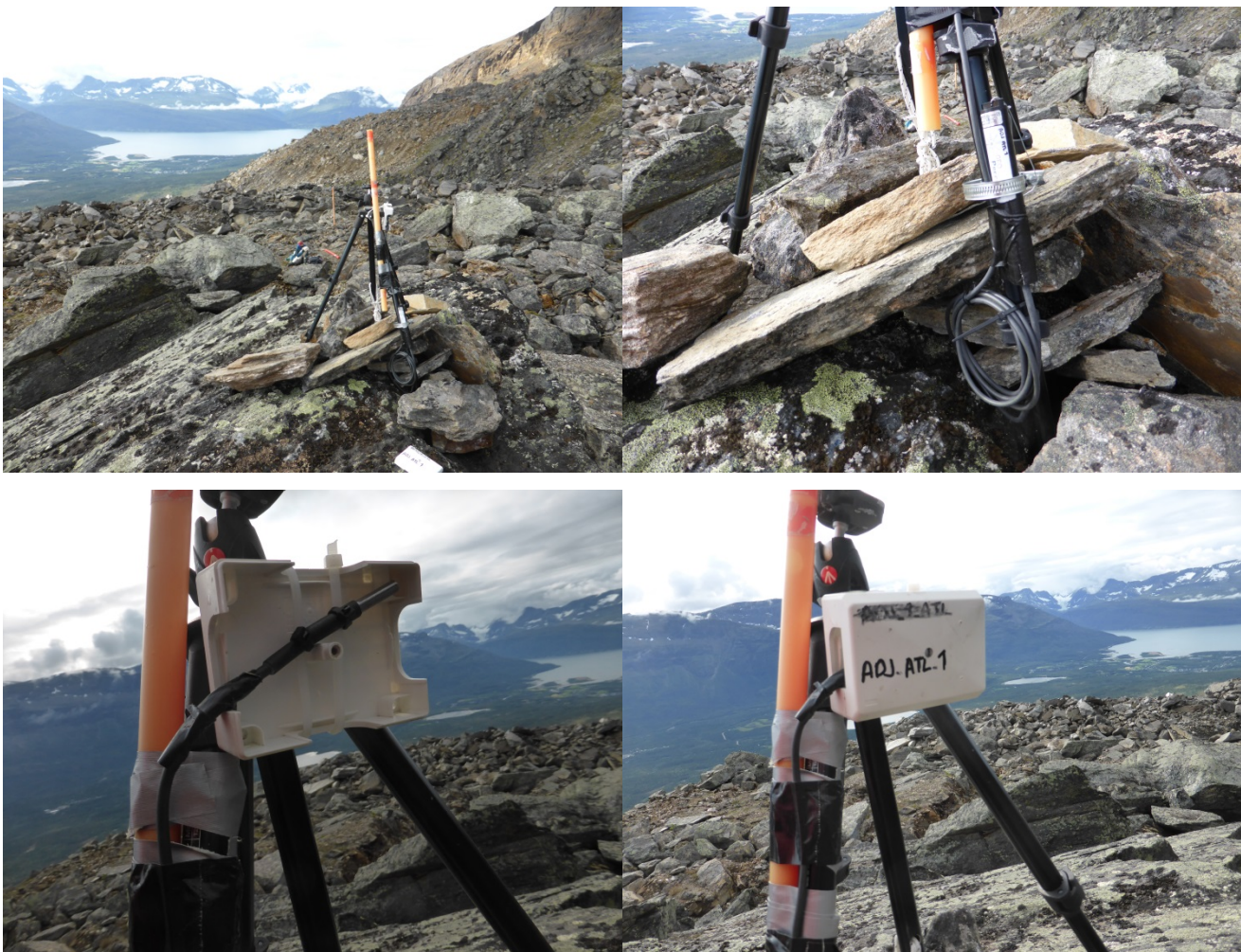
Figure 20 – ATL 1_2016 measuring air temperature on top of a large boulder in the middle part of the SE-rock glacier lobe
