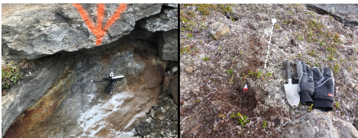
Figure 3 – Examples of mounting GeoPrecision loggers with cable (M-Log5W-CABLE) measuring temperature in a shallow borehole in a rock wall (left) and without cable measuring ground surface temperature inside a plastic stick (right).
