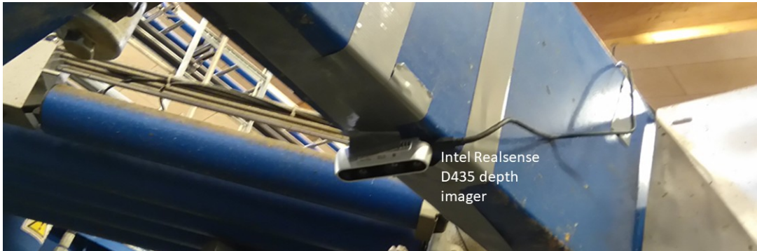
Figure 2.2: RGB-D(depth)for 3D model reconstruction of back and neck of the cattle while getting milked in the milking robot.
