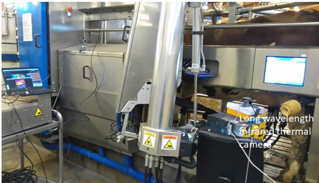
Figure 2.6: Long wavelength infrared thermal camera for udder surface temperature field imaging while the cattle get milked in the milking robot.
