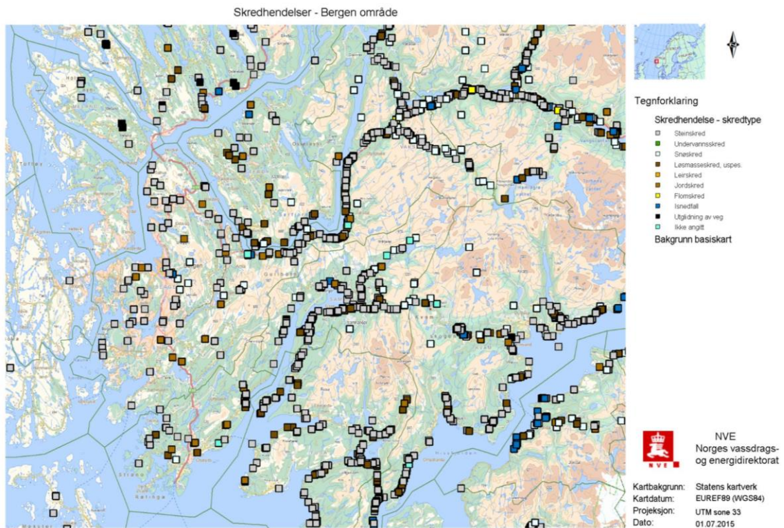
Figure 20: Extract of the inventory of natural hazards events in Norway: rockfalls (gray), landslides (brown), debris flows (yellow), roads deterioration (black), avalanches (white), icefalls (dark blue), unspecified (turquoise). From www.skrednett.no (download: 07-01-2015).
