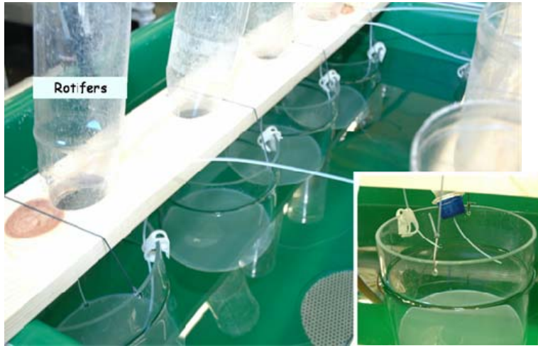
Figure 2. Experimental design/test chambers for cod larvae. Note the bottles used for feeding rotifers to the cod larvae in Exp. 1.
