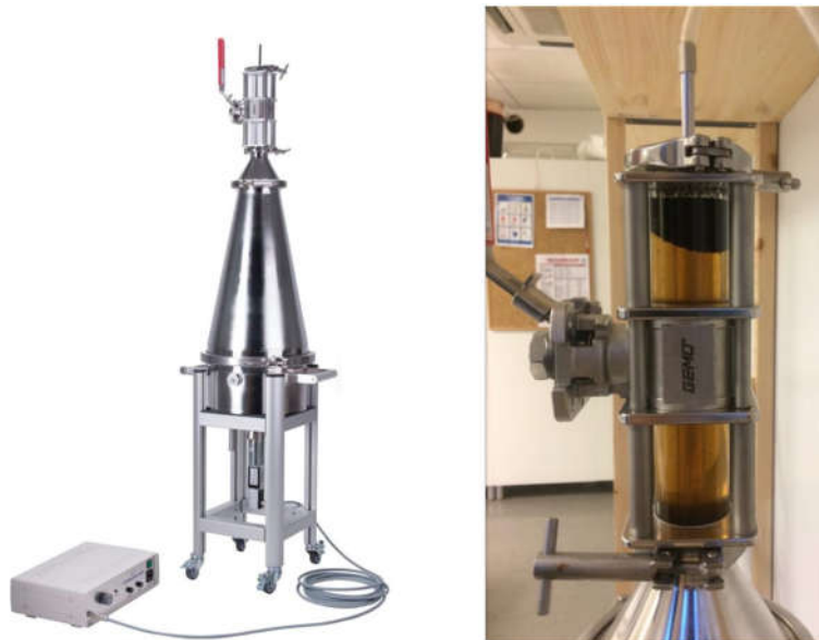
Figure 2.18 - Micro-Plastic Sediment Separator (Hydrobios, Germany) used to extract microplastics from the collected sediments (Left). Detail of the top chamber with the extracted sample (Right, photo: NORCE).
