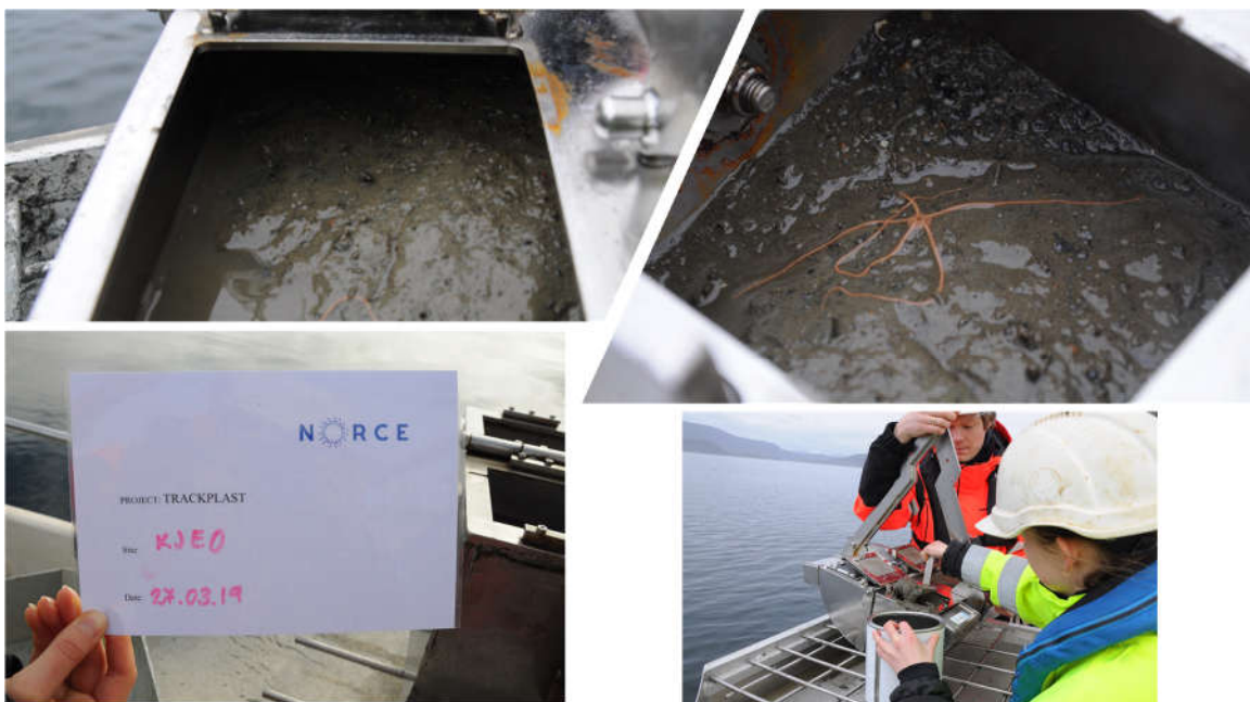
Figure 2.10 - Photos of sediments collected from a van Veen grab using a flat stainless steel sampling spoon. The top 0-5 cm of the sediment were collected in a metal container.
