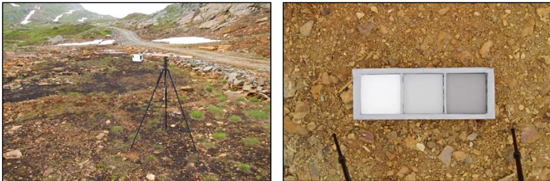
Figure 3. Set-up for in situ hyperspectral measurements with Rikola camera (left). Reflectance calibration panels (right).
