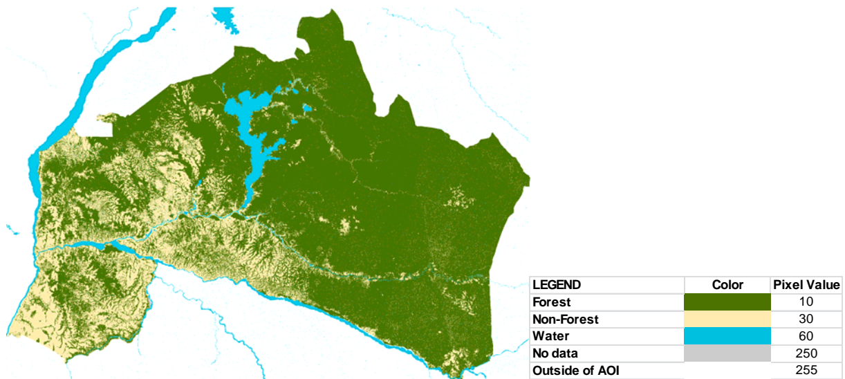
Figure 25. FNF using the four averaged backscatters features from ALOS-2 PALSAR-2 2014-2016 ( HH_{mean} , HV_{mean} ) and Sentinel-1A 2015-2016 ( VV_{mean} and VH_{mean} ).
