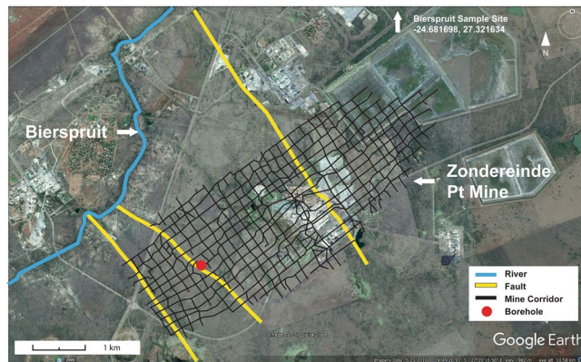
Figure 2. Zondereinde-Bierspruit system. Google Earth image of Western Bushveld Igneous Complex mining region and mining map of Zondereinde juxtaposed upon it. Black lines demarcate mine property, stopes and tunnels. Dykes strike SE-NW and faults (yellow lines) strike N-S and ESE-WSW. The borehole (red dot) lies directly on the fault leading to the Bierspruit River. Scale bar 1 km. Map data: Google, Digitalglobe.
