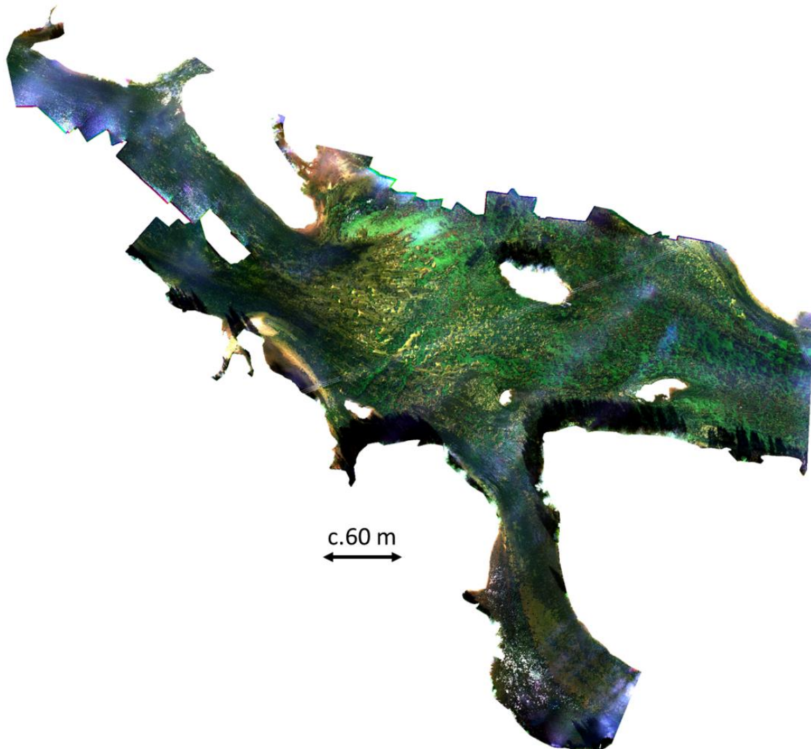
Figur 16 Area1 MicaSense RedEdge mosaic. Bands Red, Green and Blue visualised in RGB. Areas outside the riverbed is masked for improved visualisation.
