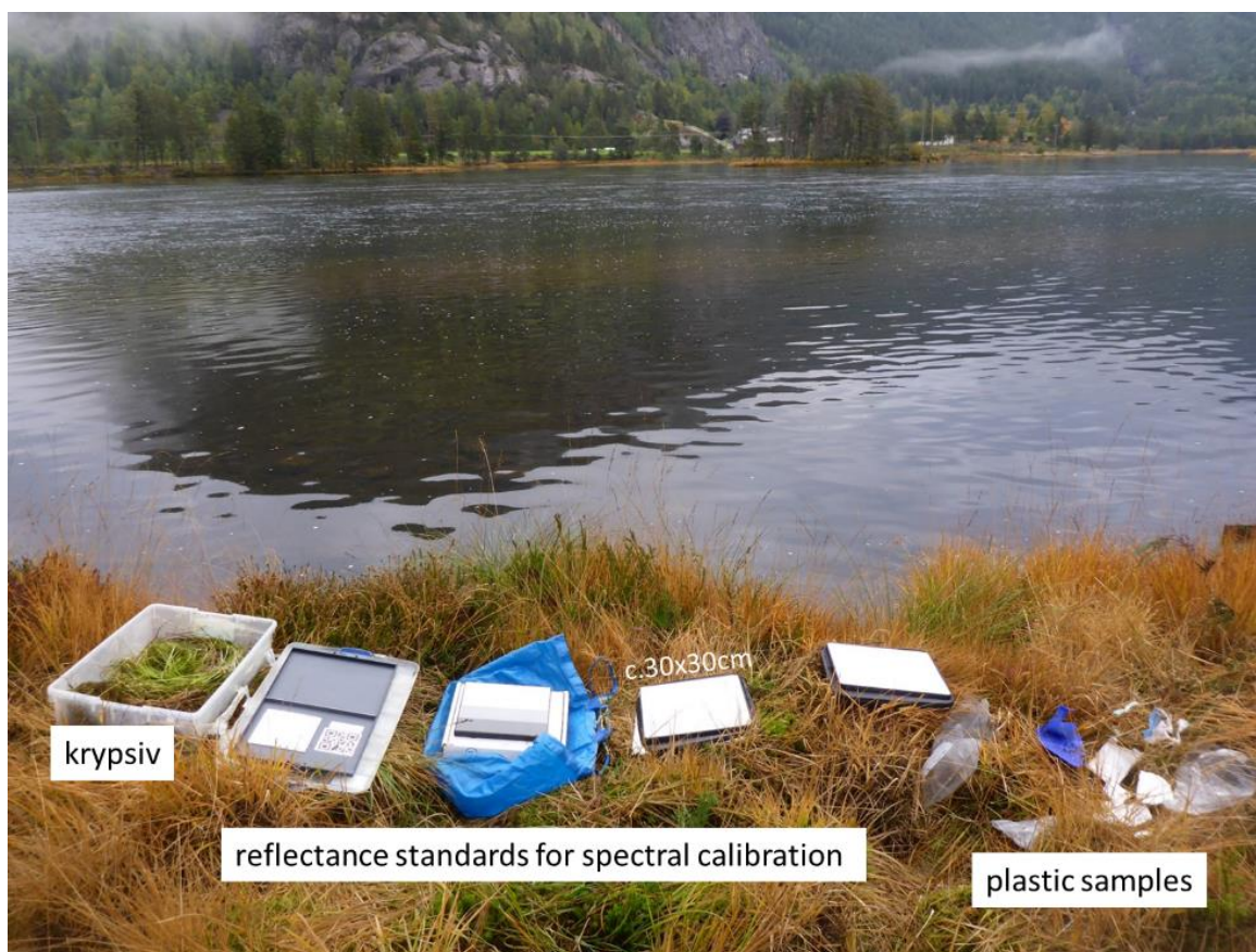
Figur 13. Calibration targets and reference material as used for multispectral imaging, shown from area 1. Some plastic material was placed and scanned as reference material to allow method assessment for plastic mapping from drones in other pilot projects.
