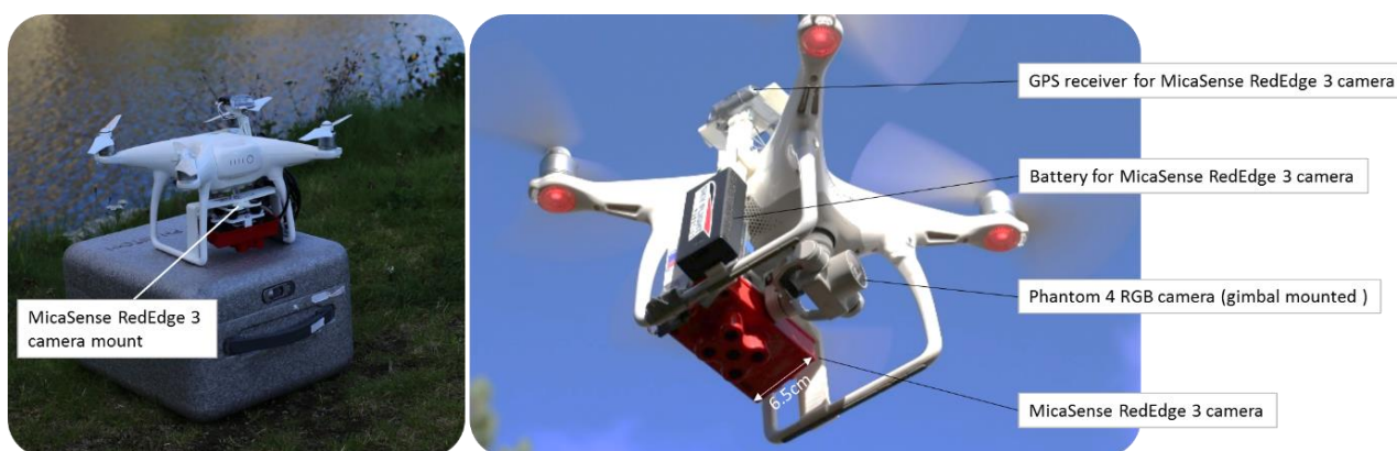
Figur 12. MicaSense RedEdge 3 camera mounted at a DJI Phantom 4.
