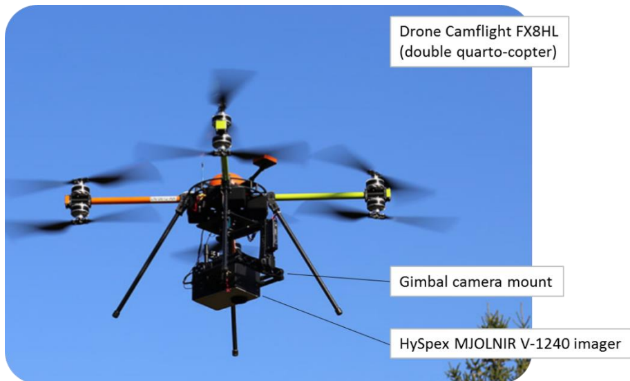
Figur 28 HySpex MJOLNIR V-1240 pushbroom camera mounted on a Camflight FX8HL drone.
