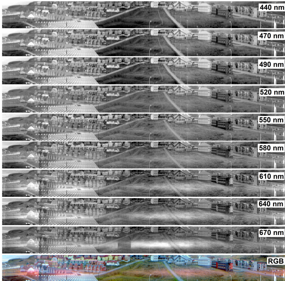
Fig. 10. Sample images from the 3D printed push broom Hyper Spectral Imager (HSI) - instrument (B). Location is at the roof of the University Centre in Svalbard (UNIS) on the 25th of September 2017. Vertical center line of the images is towards South - up the Longyearbyen valley. Each image is labeled with the center wavelength to the right. The individual images have a bandpass of 10 nm. The bottom RGB composite is constructed by combining images at center wavelengths 480 nm (blue), 550 nm (green) and 620 nm (red).
