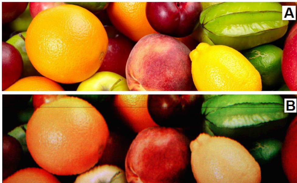
Fig. 11. Handheld gimbal operation of the push broom Hyper Spectral Imager (HSI) – instrument (B). Panel (A): Target computer screen image. Panel (B): HSI RGB composite constructed by combining center wavelength images at 490 nm (blue), 552 nm (green) and 620 nm (red). Bandpass is 10 nm for each color channel.
