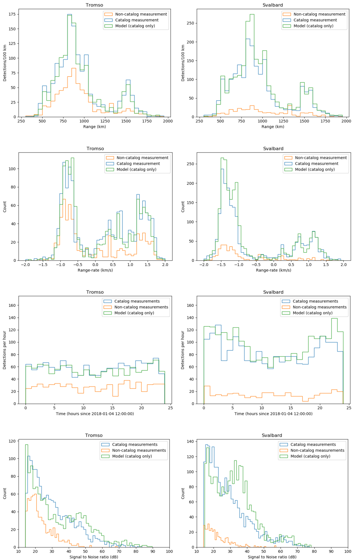
Figure 7. Histograms of detections for Tromsø (left) and Svalbard (right). Top: range histogram, second from top:
