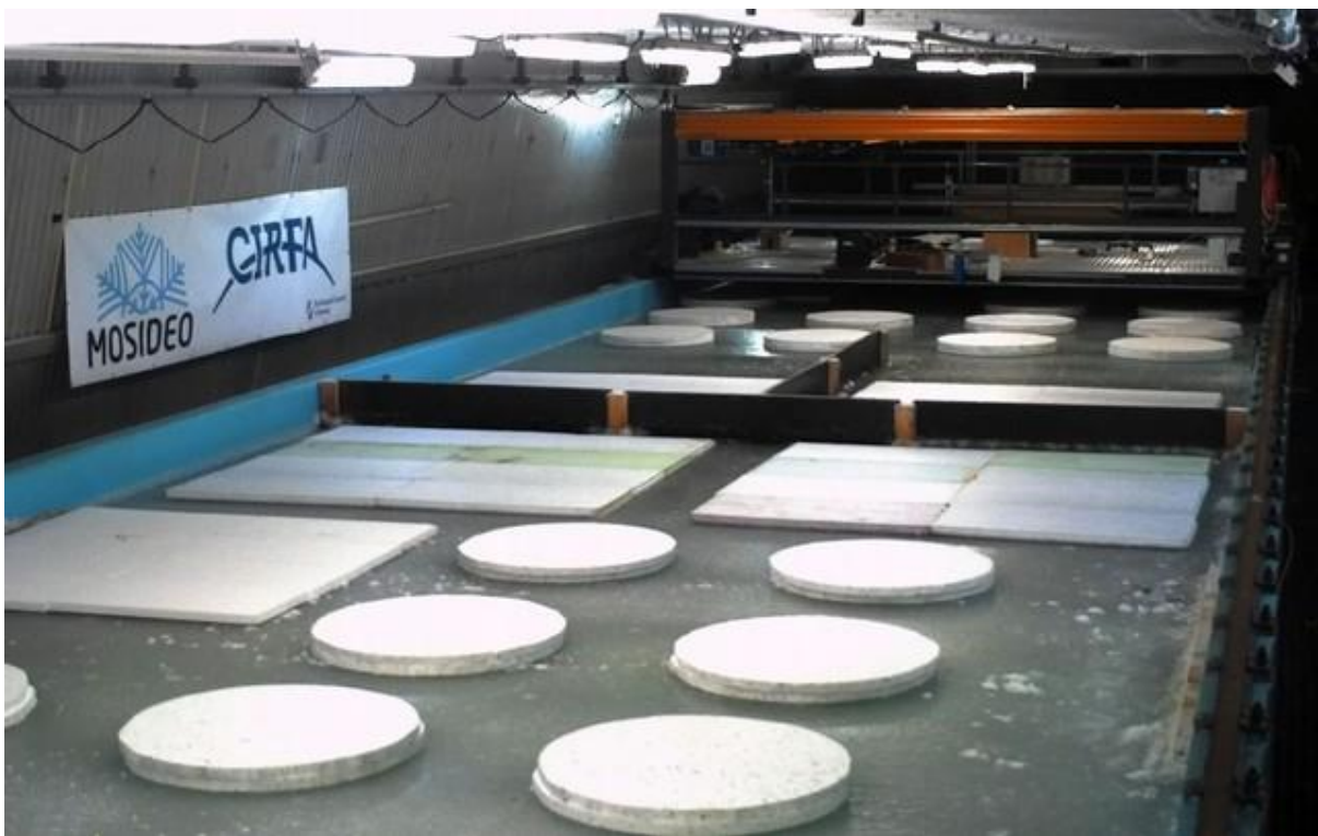
Figure 4. Surface insulation to create an under-ice profile.
