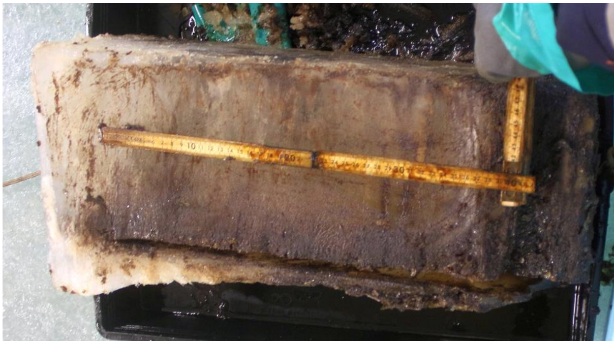
Figure 8. Example excavated medium-sized oil lens immediately after excavation. The transition to the host ice and center of the lens is seen on the left and right hand side, respectively. Also visible is the thickening of the ice beneath the oil lens toward the edge of the lens (left hand side in photo).
