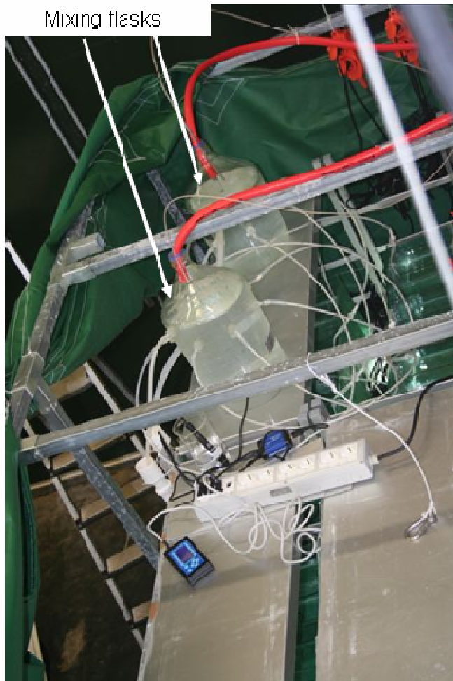
Figure 5. The mixing flasks where seawater and 5 mg/L oil dispersion is mixed to make 0.010 mg/L and 0.015 mg/L oil.
